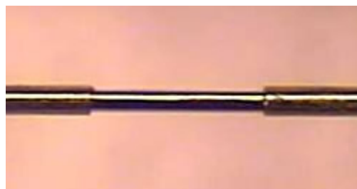
Excimer laser wire stripping; a single 50um wire, with polyimide insulation.
