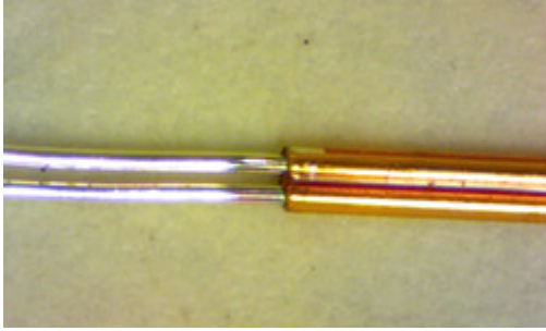
Bifilar solid core wires, 0.014" wire diameter, 0.003" thickness insulation, stripped with an IMPACT TEA CO2 laser
